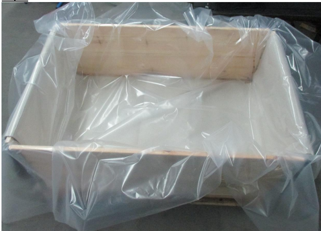
Step 3: The wooden crate is lined with film
