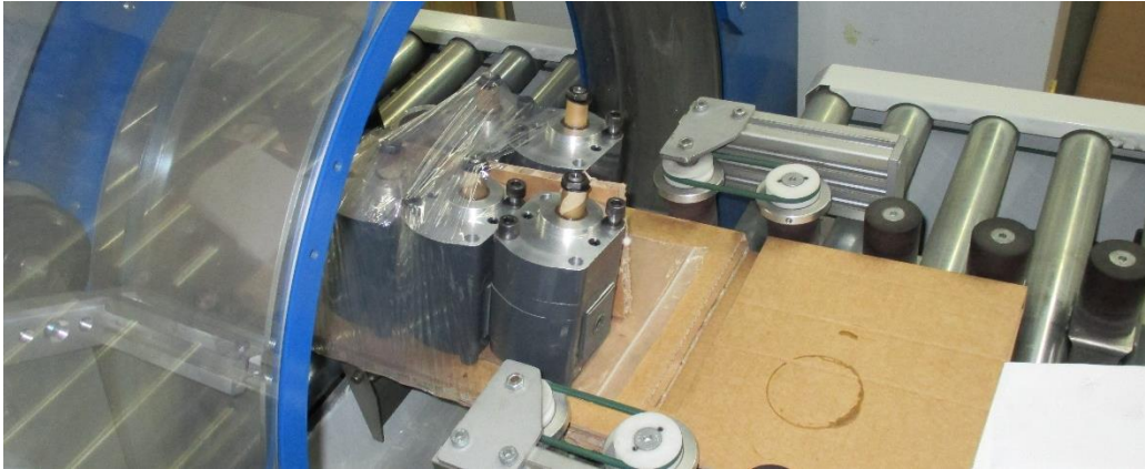
Step 2b: Fixation of the products on the inlay by strapping with stretch film
