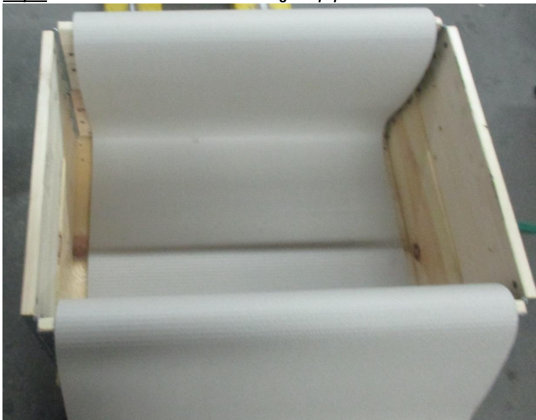
Step 2: The wooden crate is lined with corrugated paper
