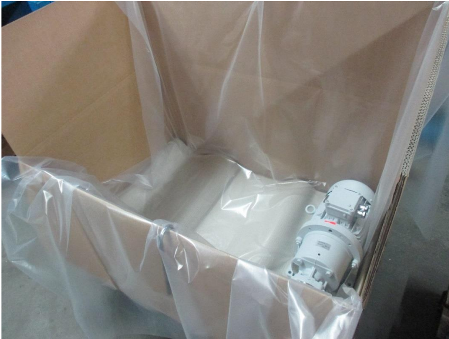
Fig. 3: Euro pallet with pallet box, sealed with PE film
