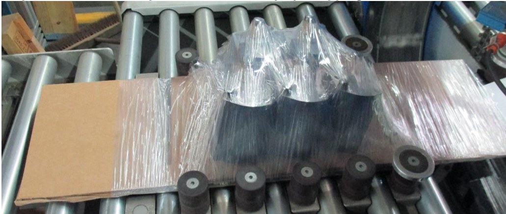
Step 2c: Fixation of the products on the inlay by strapping with stretch film
