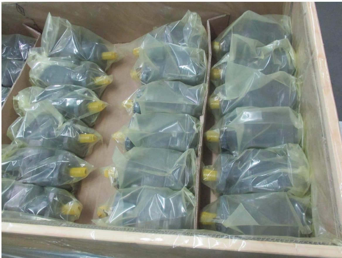
Fig. 7: Products in corrosion protection bags (VCI bag)
