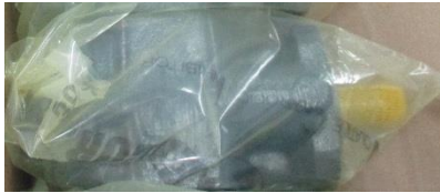
Fig. 5: Pump in a VCI bag
